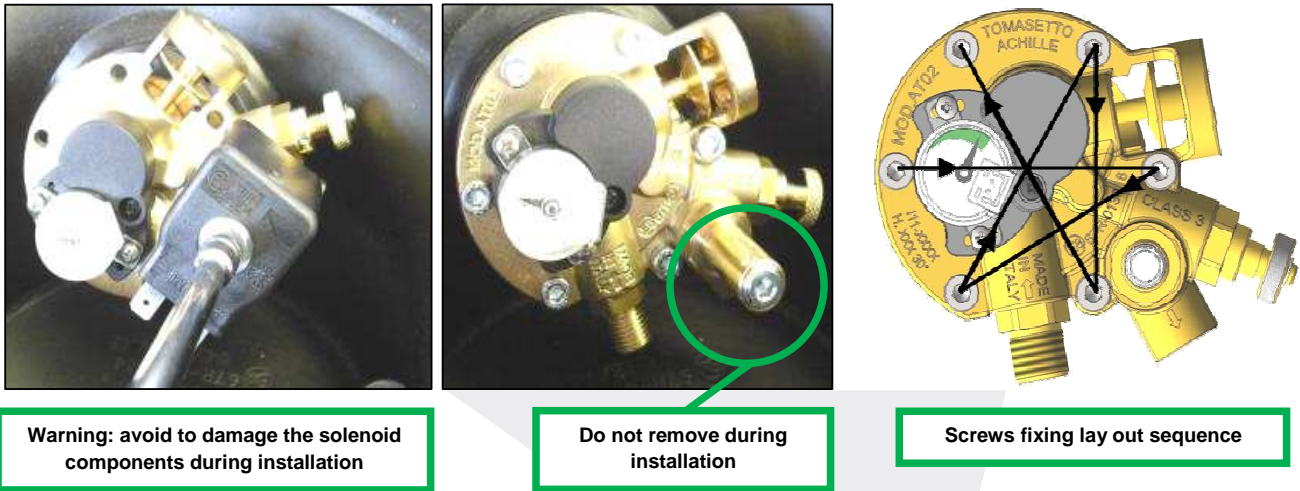
Figure 14: operation sequence for screws fixing
