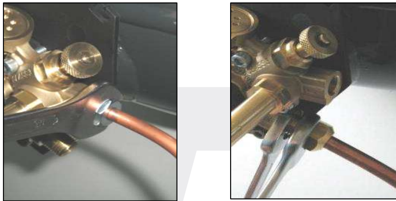
Figure 37: inlet and outlet fittings screwing 0° toroidal tank
