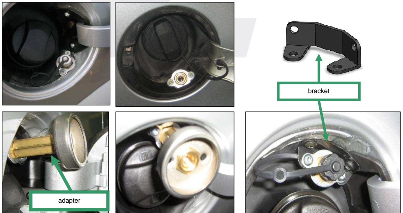
Figure 39: filling point installation
