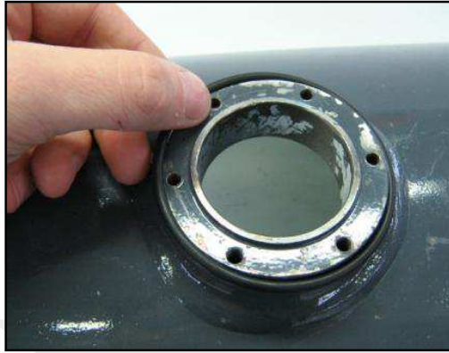
Figure 11: Placement of the O-ring gasket
