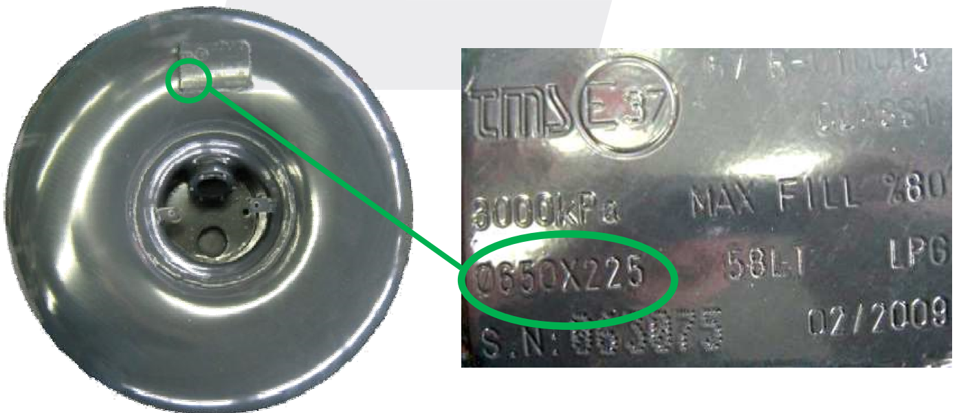
Figure 2: LPG tank size
