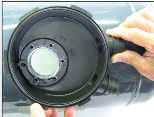
Figure 12: Positioning of the gas tight housing
