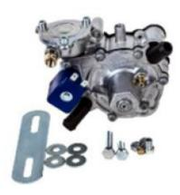
The **EN09N** reducers, the latest evolution of the EN09 sequential reducers family, has been designed with the aim of further improving the performance compared to the other reducers of the EN09 family, thanks to the improved heating circuit and the higher support engines power, up to 125kW. This reducer differs on the integral body, the complete separation of the water and gas circuits, the improved gas circuit and the deeper water circuit,
