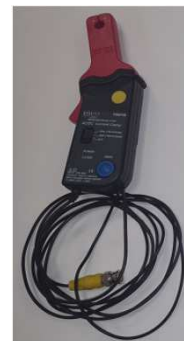
20 A / 60 A DC (low amps) current clamp 1 mV/10 mA (100 mV = 1 A) — use this for testing currents up to 20 A. 1 mV/100 mA (10 mV = 1 A) — use this for testing current up to 60 A. Code TA018
