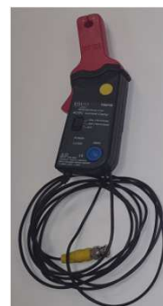
20 A / 60 A DC (basso amperaggio) pinza di corrente 1 mV/10 mA (100 mV = 1 A) — use this for testing currents up to 20 A. 1 mV/100 mA (10 mV = 1 A) — use this for testing current up to 60 A. Codice TA018
