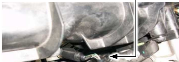
8 (OR 10) PIN PETROL INJECTORS CONNECTOR
